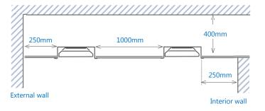
Note. When recessing into a T-tail grid ceiling, an proprietary accessory bridging bracket is required.
