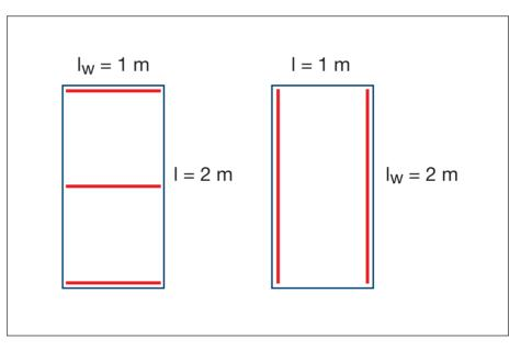
As we can see from this example, the length of a devifast<sup>™</sup> fitting band may vary although the area and the distance between the devifast fitting bands remain the same
